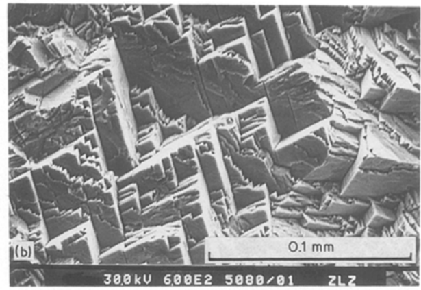
Figure 10 (a, b) SEM micrographs showing the fatigue fracture appearance of coarse dendritic structure cast Co-Cr-Mo alloy. Faceted growth and stepwise cleavage fractures following crystallographic planes.
