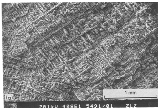
Figure 7 (a, b) SEM micrographs showing the tensile fracture appearance of the dendritic structure in cast Co-Cr-Mo alloy.
